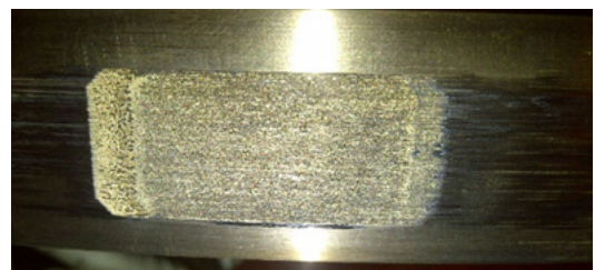
Figure 1: Photographing or ghosting on a slip ring
